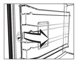
■ Pull the runner out of the front fixing to release it.
